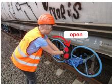
It is difficult to open the wagons when loaded as the dimensions of the unloading hopper are much larger than on smaller wagons and the entire weight of cargo lies on these hoppers. Therefore, the pressure on the opening is really considerable.
