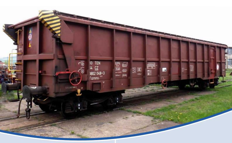
4 – axle high-walled cargo wagon with an opening roof
